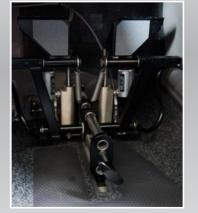
Electrically Operated Adjustable Rudder Pedals for Pilot and Copilot
