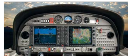
GARMIN G1000 COCKPIT: DA42-VI, DA42 NG + DA40 NG Advanced avionics system
